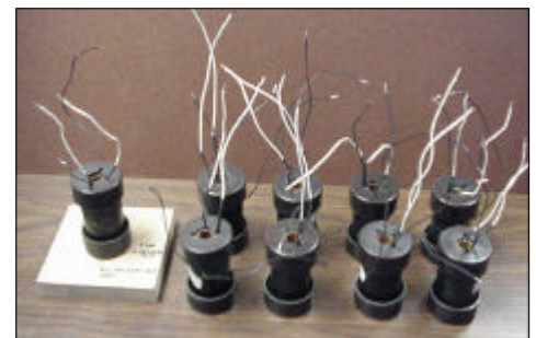
Coils potted using jig.
