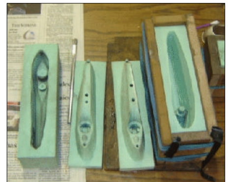
Metal casting moulds for Metropolitan door handle
