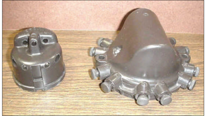
Our most complicated cap to date was the 6-cylinder Lucas cap. It dwarfs in comparison to the Liberty pattern distributor cap.
