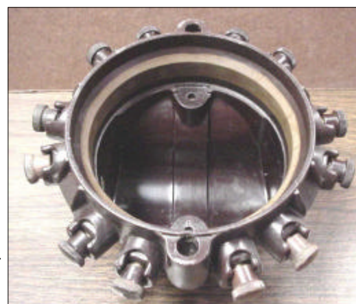
The original pattern Liberty distributor cap. Note the asbestos high tension ring.
