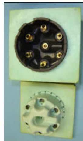
Sample of a reproduction distributor cap. Made in small batches, caps are concourse quality.
