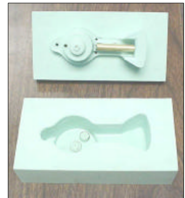
Open Liberty Distributor Rotor Mould
