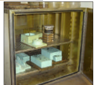
Moulds ready after baking (left).
