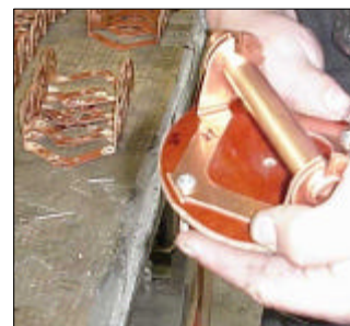
Coil Baseplate Fabrication and Assembly
