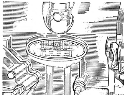
The Automatic Transmission Number is stamped on a plate secured to the left-hand side of the transmission casing
